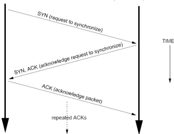
The Three-way TCP Handshake for a reliable communication.
