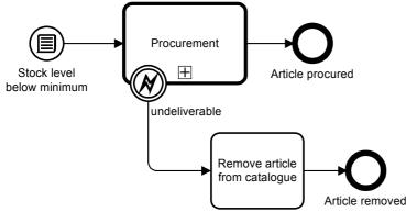
Figure 5.4: Stock maintenance process
